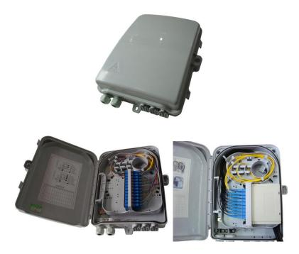
This terminal box terminates up to 2 fiber optic cables, offers spaces for splitters and up to 48 fusions, allocates 24 SC adapters and working under both indoor and outdoor environments. It is a perfect cost-effective solution-provider in the FTTx networks.
