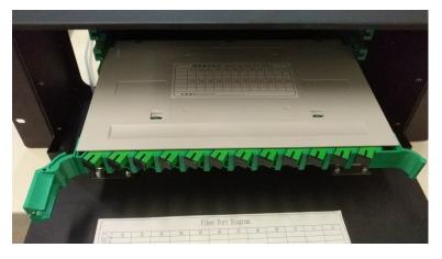
8. Remove the tray cover. Insert the fibers into the tray from the cable entrance on the left or right sides of the tray. Fix the protection tube with a cable tie.
